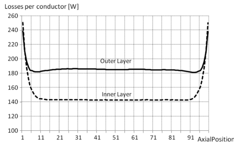
Fig. 3. Rated total losses per conductor in the LV winding.
